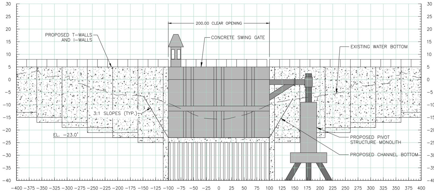
**FRESHWATER BAYOU BY-PASS CONCRETE BARGE TYPICAL SECTION**
