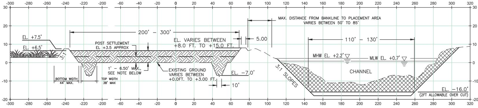
**COMMERCIAL CANAL TYPICAL PLACEMENT SECTION**
